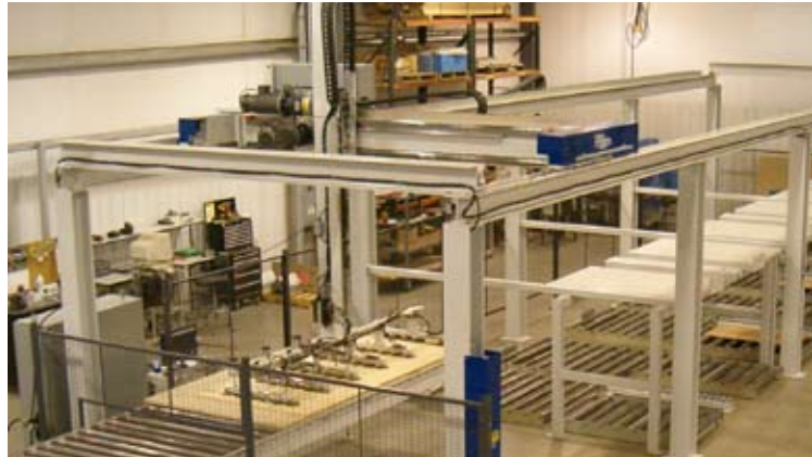
Shown is an overhead view of the material sorting system at Northway Industries that incorporates special vacuum cups for moving panels.
